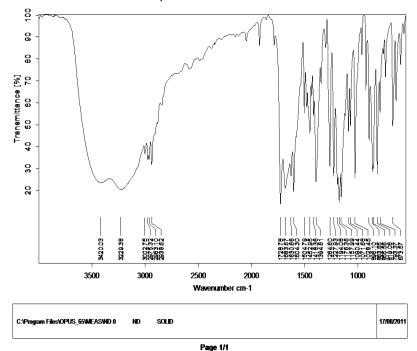
Figure 4: FTIR graph of pure drug (Naproxen)
