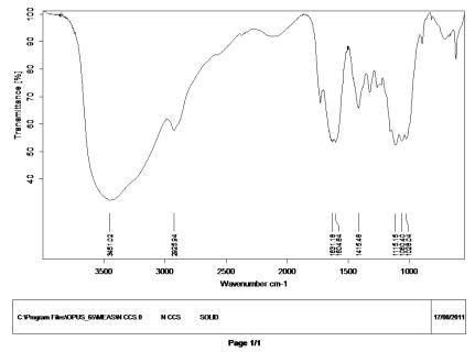
Figure 6: FTIR graph of Croscarmellose sodium
