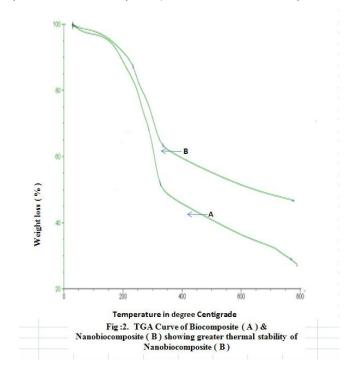
**Kinetic study of thermal degradation reaction :** The order of reaction and activation energy of thermal degradation reaction for the composite and Nanocomposites were calculated from thermochemical data using Friedman technique<sup>[23]</sup> and is represented in **Table(4)**. The order of reaction is as expected, since it is a well known fact that the decomposition of copolymers do not obey first order kinetic perfectly<sup>.[24]</sup>
