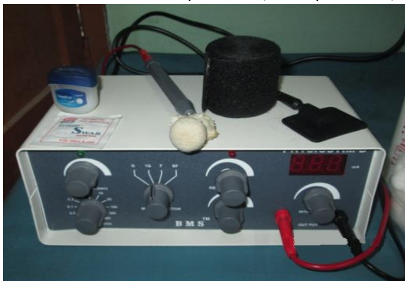
Fig -1 Electrical stimulator with active pen electrode, inactive pad electrode, strap, gel.
