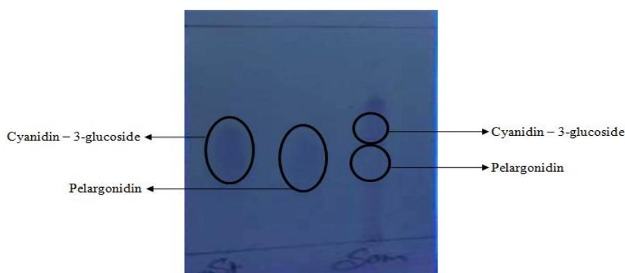
**Figure 1. TLC separation of Red tamarind unripe fruit extract**
