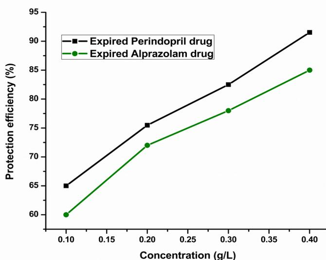
**Figure 2: Protection efficiency of the corrosion inhibitors with four different amounts**
