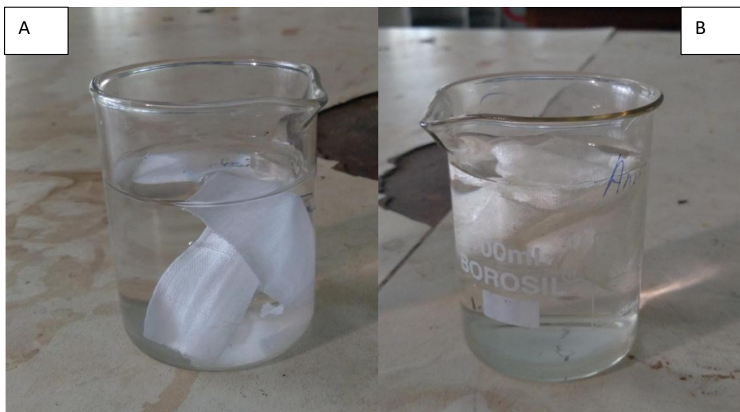
Figure3 A and B: Before scouring and After scouring.
