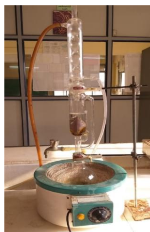
Figure No.01: Soxhlet extraction
