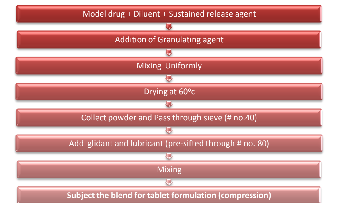
Figure No: 1 Representation of Wet granulation Technique for design of sustained release tablet
