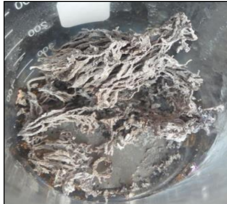
Fig 1: Cluster of hairs form of the synthesized carbon-coated cobalt nanoparticles.
