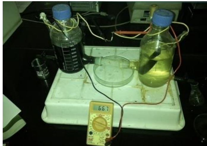
Plate 1: A model MFCs set used during current research
