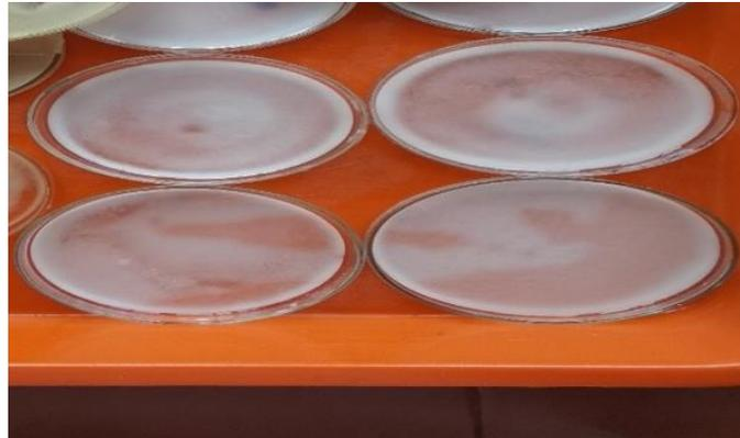
Fig 1: Bioplastic from cassava starch
