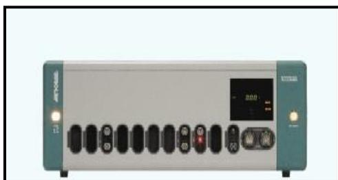
Electrochemical workstation- PG STAT 30 with 663 VA Electrode stand (Metrohm)
